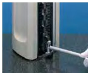
Using height master to set bore gage
