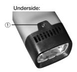
E1: Front bezel is not fastened correctly. If the E1 message appears, the instrument must be switched off. Remove the front bezel screw, reseat the reflector and tighten the front bezel screw (①).
