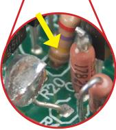
Twist the thermistor away from the resistor, or cut it out completely. Note the absence of the connection, identified by the yellow arrow. Then, install the new battery and reassemble the two halves of the housing.
