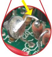
Identify the R4 resistor (brown color), with the thermistor (silver color) soldered to it. The connection between the two components is highlighted with a yellow arrow.
