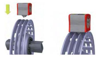
The Fixturlaser PAT units are very easily mounted on the pulleys. The spring action probe finds the center of the belt groove. The industrial built-in magnets snap the units to the pulley in a perfect fit.
