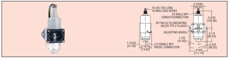
Same rugged construction as used in Series 1000W plus explosion-proof design are combined in this new unit. UL listed for Class I, Groups A, B, C & D; Class II, Groups E, F & G. Bellville spring movement permits mounting of control in any position and helps prevent contact chatter. High over-pressure protection and vibration resistance are also featured.
