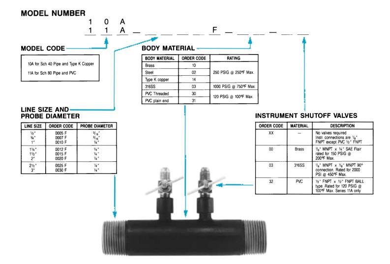
SERIES 10A inline sensors are supplied in threaded Schedule 40 pipe nipples (except for the type "K" Copper). The inline sensor is complete with factory-fitted probes and is supplied as a complete assembly providing for economical installation. Series 10A sensors are supplied with Steel, 316SS, Brass, and Type "K" copper. Available in line sizes ½" through 3".
