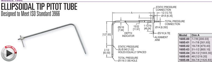
The **Series 160E Ellipsoidal Tip Pitot Tube** uses a precision crafted tip configuration, which allows air to pass smoothly with minimum turbulence for consistent, reliable readings. Sliding depth indicators grip firmly to ensure uniform insertion when measuring traverses across ducts. Total and static pressure taps are  $1/4^{\prime\prime}$  (6 mm) and are permanently silver soldered to the connection block, making them leak-proof and durable.
