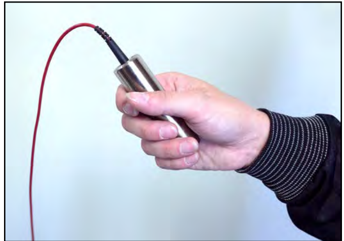
Figure 11. Using the Desco 19295 Handheld Electrode
