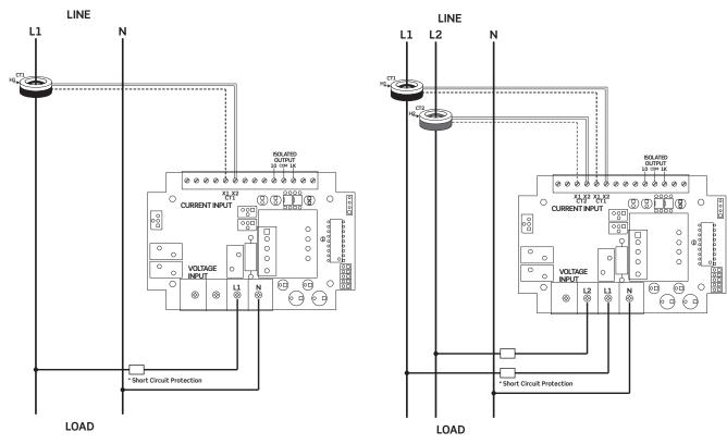
Leviton recommends solid core transformers (CTs) for revenue-grade accuracy. Our 100A and 200A color coded CTs assist with correct installation by indicating phase monitored. Split core CTs are also available upon request for applications where power cannot be interrupted during installation. Our 100-800 Amp Split Core CTs offer +/-1.0% accuracy.
