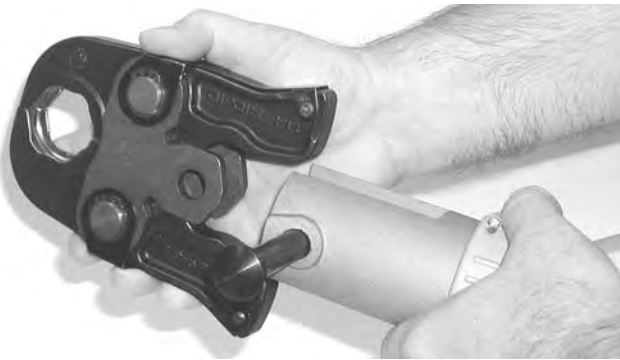
Figure 5 – Pulling The Jaw Set Mounting Pin Out
