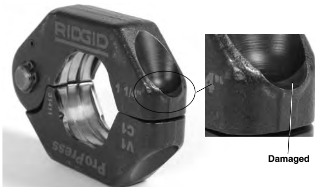
Figure 13 – Damaged Ring Pocket
