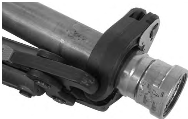
Figure 14B – Placing V2 Actuator Into XL-C Ring Pockets At An Angle For Additional Clearance
