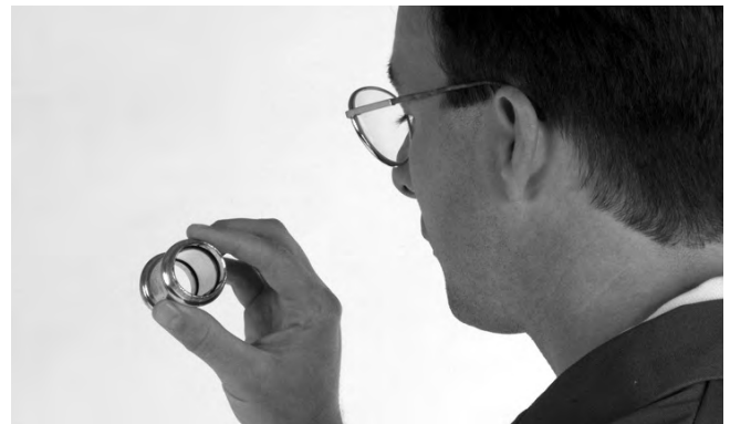
Figure 6A – Inspection of the ProPress Fitting per the Manufacturer's Instructions
