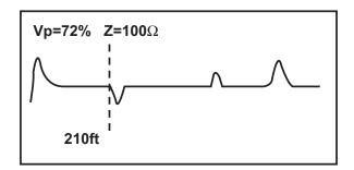
The vertical cursor line is moved left and right along the line of the trace by pressing the ◀ and ▶ buttons.
