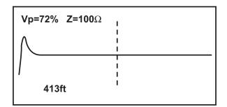
The following display shows a cable with impedance anomalies on it.
