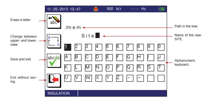
You can then rename the SITE. Start by erasing the existing text. Then move about on the keyboard using the directional keypad (  $\blacktriangle \nabla \blacktriangleleft \blacktriangleright$  ) and validate each letter by pressing the **OK** key.
