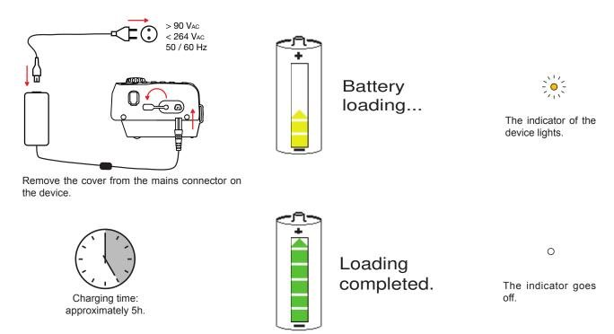
Set the switch to OFF, but charging is possible when the device is not off.
