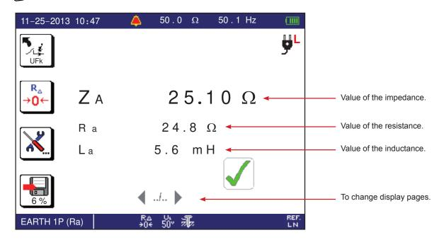
The third page displays the values of  $Z_s$ ,  $R_s$ ,  $L_s$ . The fourth page displays the voltages  $U_{l,N}$ ,  $U_{l,PF}$ ,  $U_{NPF}$  and on the rod ( $\longrightarrow$ ) before the measurement.
