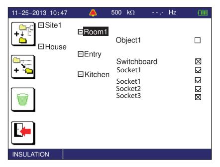
Press the key to erase ROOM1. The device asks you to confirm by pressing the **OK** key or abort by pressing the key.
