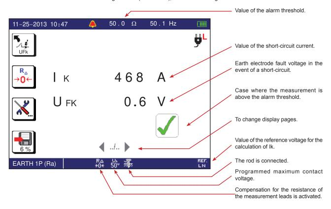
$U_{Fk}$  is calculated only in earth measurement on live circuit with a high current (TRIP mode).  $U_{Fk}$  = Ik x  $Z_A$ .
