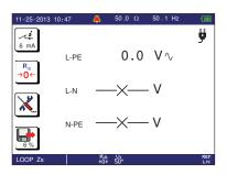
If  $U_{\text{N-PE}}$  does not display -x --, the protection in the N terminal has been activated.
