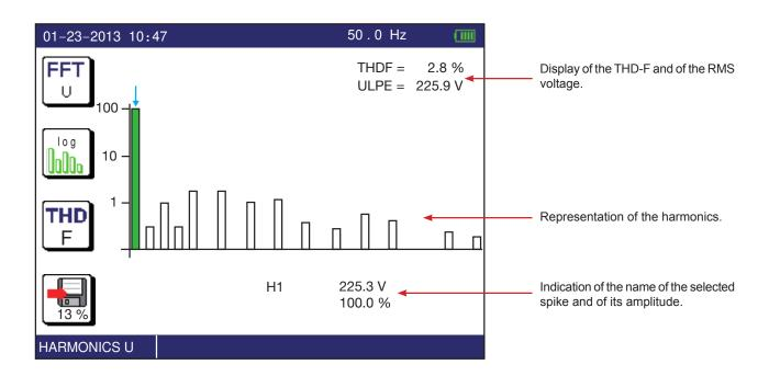
The frequency and amplitude of the selected harmonic (in black) are indicated at the bottom of the graph. To select another harmonic, use the ◀ ► keys. The device then shifts from the fundamental (H1) to harmonic H2, then to harmonics (H3, H4, ..., H25). And on the next page it sweeps the harmonics from H26 to H50.
