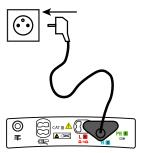
In the Zs (RA/SEL) and RCD, settings, the device also indicates the position of the phase on the display unit using the symbol. The mains socket outlet of the measuring cable is marked with a white reference spot.
