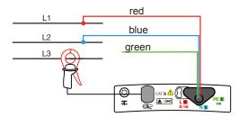
The power measurement can be made on different phases of an installation. This is why it has been made possible to index the recorded power value with one of the following values: 1, 2, or 3 (single-phase measurements on a three-phase network).
