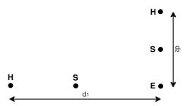
If you find the same values, your measurement is reliable. If the measured values are substantially different, it is probable that they were influenced by earth currents or a groundwater artery. It may be useful to drive the rods deeper.
