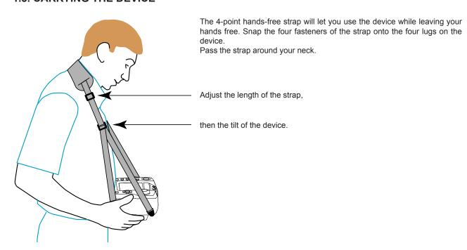
To withdraw the strap, slide a flat screwdriver under the tab of the fastener to lift it, then slide the fastener down.
