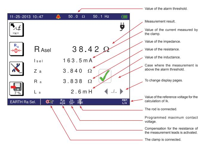
The second page is used to see the value of short-circuit current lk, f loop impedance Z<sub>e</sub>, of loop resistance R<sub>e</sub> and of loop inductance L<sub>s</sub>.
