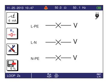
If  $U_{\text{L-PE}}$  does not display – x --, the protection in the L terminal has been activated.
