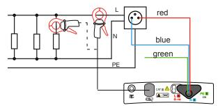
In the case of a three-phase network balanced in voltage and in current, connect the measuring cable terminated by 3 leads to the device and to two of the three voltages  $U_{12}$ ,  $U_{23}$  or  $U_{31}$  using the red and green leads. Then, with the clamp, surround the conductor of the third phase  $I_3$  (for  $U_{12}$ ),  $I_4$  (for  $U_{23}$ ) or  $I_2$  (for  $U_{31}$ ).
