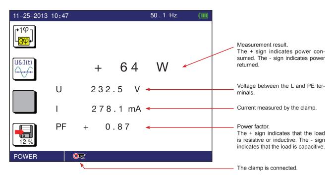
If the phase of the current with respect to the voltage is not correct, turn the clamp around, with the help of the arrow marked on the jaws, in order to reverse the phase by 180°.
