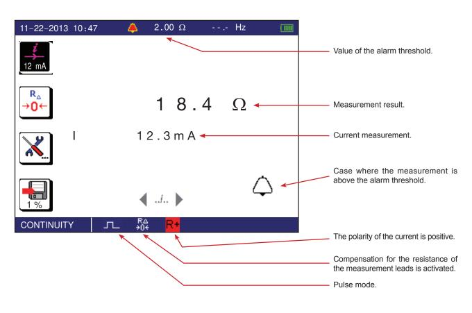
■ In the case of a resistance measurement (kΩ), there is no current reversal and no compensation for the measurement leads.
