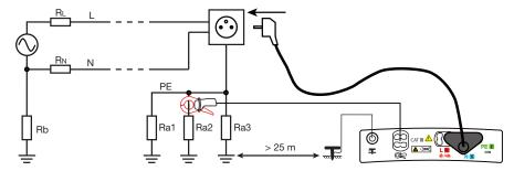
For a more accurate measurement, you can choose a high current (TRIP mode), but the RCD that protects the installation may trip.
