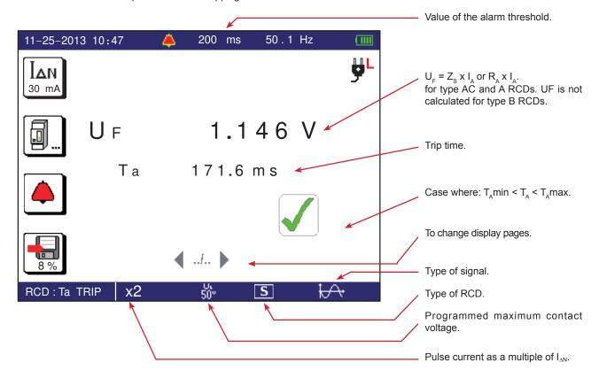
■ In the case of a non-tripping test in pulse mode:
