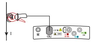
Here, the conductor passes through the clamp 4 times. You will have to divide the measured current by 4 to know the true value of  ${\sf I}$ .
