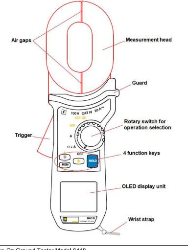
Clamp-On Ground Tester Model 6418
