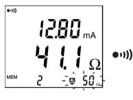
The alarm indicator on the display blinks and the instrument emits a continuous audible signal.
