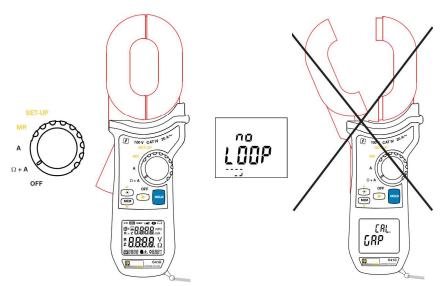
If the instrument fails to complete self-calibration, the error message **Err. CAL** is displayed. If this happens, turn the instrument OFF and ensure the air gaps are clean. Then turn the instrument ON.
