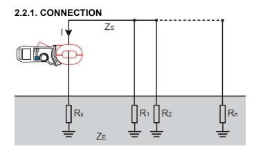
The ground electrode to be measured (R<sub>x</sub>) is in a series/parallel arrangement with other ground electrodes via the earth impedance (Z<sub>E</sub>) and physical connection to other resistance paths (Z<sub>S</sub>). The measured impedance will be slightly greater than R<sub>x</sub> assuming the downstream impedance is very low. For example: If R<sub>x</sub> is 21Ω and Z<sub>S</sub>/R<sub>1</sub>-R<sub>n</sub> is effectively 0.6Ω, the Model 6418 will read 21.6Ω.
