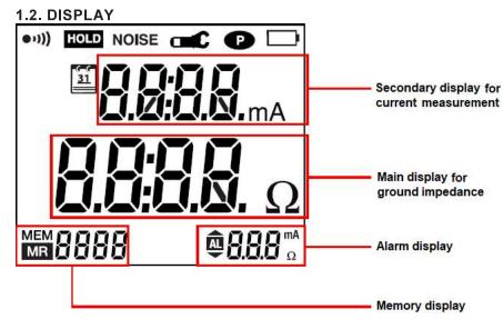
When the measurement exceeds the limits of the measurement range, the instrument displays **OR**.
