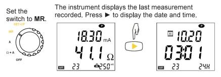
Use  $\blacktriangle$  and  $\triangledown$  to scroll through all of the recorded measurements.
