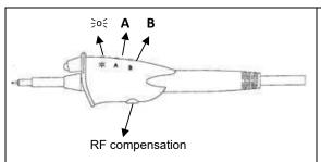
The *HX0030* probe has three directly accessible control buttons:
