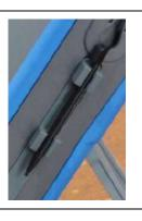
The stylus is stored in the holder on the side of the instrument.
