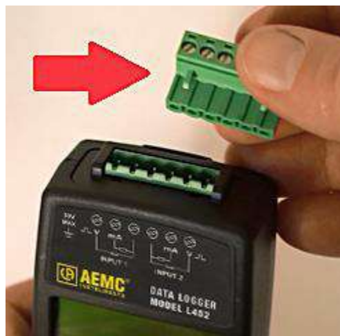
Figure 23. Terminal strip (upper right)
