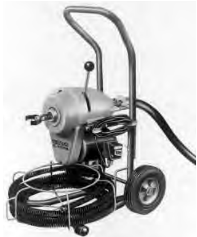
Figure 11 – Storing Cables On "A" Frame Models
