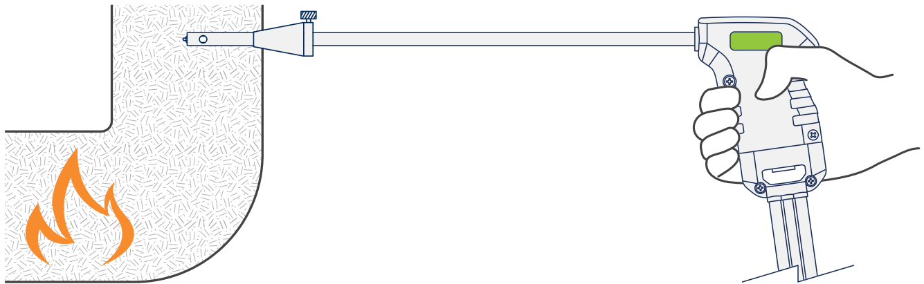
Fig. 3-6: Probe Placed in Center of Measurement Area
