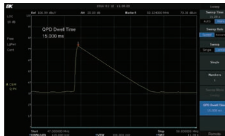
Quasi-peak detection with dwell time helps identify non-compliant emissions.
