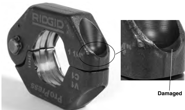
Figure 13 – Damaged Ring Pocket
