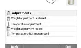
Press the Weight and temperature adjustment button to access the adjustment screen.
