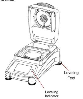
Adjust the leveling feet of the Moisture Analyzer until the air bubble in the indicator is centered. The level indicator is located under the cover towards the rear of the Moisture Analyzer.
