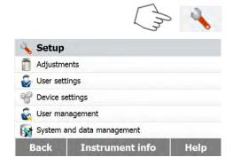
Press the **Setup** button to access Setup menu.
