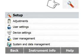
Press the Setup button to access the Setup menu.
