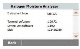
You can view **Instrument type**, **Terminal Software**, **Drying unit software** and **SNR** information.
