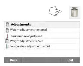
Press the Weight and temperature adjustment button to access adjustment menu.
