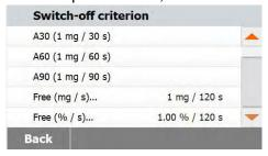
Select **Free (mg / s)** means weight loss per unit of time.
