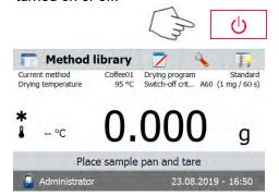
The **Moisture Analyzer** turns on automatically when connected to a power source. An internal diagnostic test is performed; the display lights and the Home screen appears followed by the initial display.
