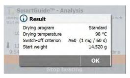
When the process is finished, the **SmartGuide<sup>™</sup>** will provide a suggested heating method including drying program, drying temperature and switch-off criterion in the result.
