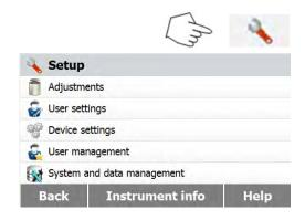
Press the Setup button to access the Setup screen.
