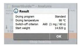
When the process is finished, the **SmartGuide<sup>TM</sup>** will provide a suggested heating method including drying program, drying temperate and switch-off criterion in the result.
