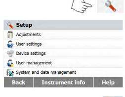
Press the **Setup** button to access the Setup menu
