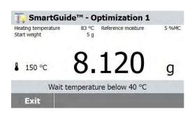
**Note:** The moisture analyzer needs to cool down if the temperature of heating chamber is above 40° C.
