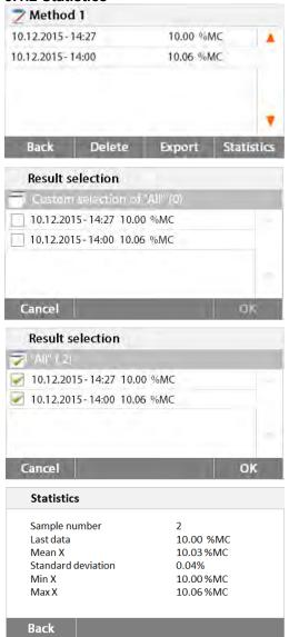
Select the method name to list all the test results of the method.
