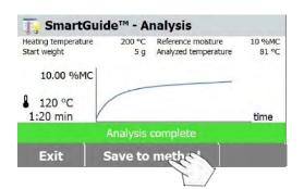
Press the **Save to method** button to save the suggested heating method to the method library for future use. EN-42 MB120
