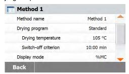
Press the **Drying Temperature** button to access the temperature setting menu.
