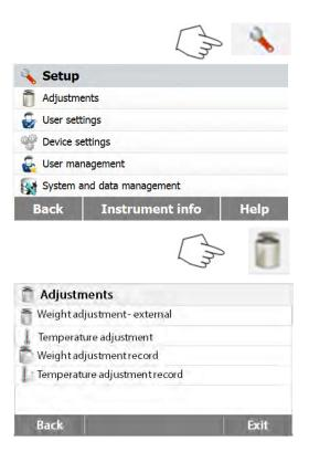
Press Setup button to access the adjustment menu.
