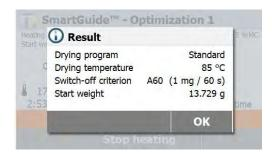
When the optimization process is finished, the **SmartGuide**<sup>™</sup> will provide an optimized heating method including drying program, drying temperate and switch-off criterion in the result.
