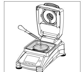
Wet the glass fiber pan with a 0.5 to 1 gram of water. Attention: Minimum sample size must be greater than 0.5 gram.
