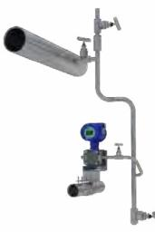
For high temperature steam measurement in a pipeline by differential pressure transmitter, pre-inject cooling water into the guided pipe. Once the steam pipes are stable, slowly open the shut-off valve and start measuring.
