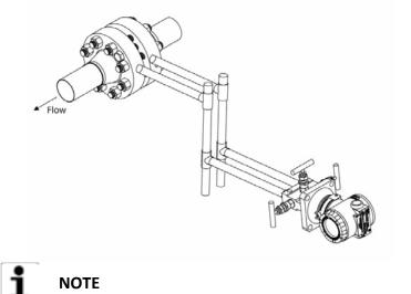
For steam or other higher temperature processes, ensure that the temperature at the process connection does not exceed the transmitter's process temperature limits.
