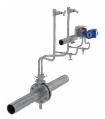
For liquid flow measurement, up-tilt the guiding pressure tube by 45°. Ensure that transmitter installation location is at lower level than that of the process pipeline. Pre-inject cooling liquid into the guiding pressure tube. Slowly open the shut-off valve to start measurement. Periodically open the drain vent to clear the residual gas from the guiding pressure tube, which will improve the measurement accuracy.
