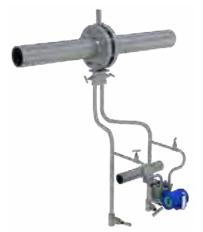
For liquid flow measurement, tilt down the guiding pressure tube by 45°. Ensure that transmitter installation location is at lower level than that of the process pipeline. Pre-inject cooling liquid into the guiding pressure tube. Slowly open the shut-off valve to start measurement. Periodically open the drain vent to clear the residual liquid, which will improve the measurement accuracy.
