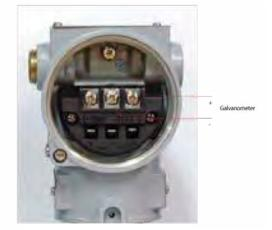
Test Terminal is marked as TEST on the terminal block. Connect TEST and negative terminal to the test terminal. Ensure that the voltage across the receptacles is kept below the diode threshold voltage so that no current passes through the diode. Make sure that the resistance of the test connection does not exceed 10 ohms while connecting an indicating meter or while taking the test readings. Note that a resistance of 30 ohms can cause an error of approximately 10% of actual value.
