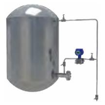
Use a single flange diaphragm system for sealed container level measurement. Increase the isolation tank and multiple shut-off valves. Periodically open the drain/vent valve to clear off the residual gas and liquid in the guiding pressure tube for higher accuracy.
