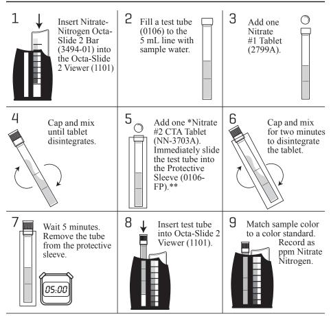
NOTE: To convert to Nitrate, multiply results by 4.4. Record as ppm Nitrate.
