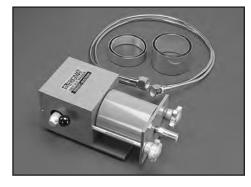
The Frigimat<sup>®</sup> Dry Ice Maker eliminates the need to buy large quantities of dry ice, producing a solid 16 ounce (454gm) block in one to two minutes. Removing the dry ice block requires just 30 seconds, and the Frigimat<sup>®</sup> Dry Ice Maker is then ready to make another block of dry ice. Each cylinder of liquid CO<sub>2</sub> will make 8 or 9 blocks of dry ice.
