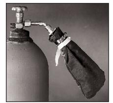
valve tightly and tap the cone gently to remove any ice sticking to it. The ice may be squeezed into a hard pack or left in flake form depending upon its intended use.
