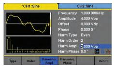
Quickly output harmonics up to the l6th order with independent amplitude and phase settings.
