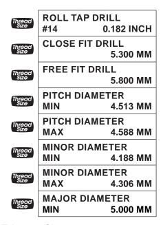
5. Switch to External 4g Tolerance Class:
