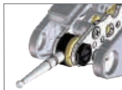
Stylus bearing screw held in sub-plate.
