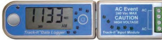
The Track-It™ AC Event Logger can also be used to record ambient temperature along with on/off cycles. This can help diagnose heat vs. cycle time issues. Information displayed on the LCD is also user programmable and can be sequenced by pressing the logger button. The multicolor LED indicator notifies the user of temperature alarms or general activity.
