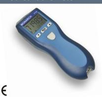
The *Pocket Tach 99 (PT99)* is a digital, battery-powered portable non-contact optical tachometer, which operates up to 36 inches from a reflective target using a bright red LED light source. The ergonomic design allows safe, direct line-of-sight viewing of both the rotating target and the display at the same time, while providing a non-slip rubber surface for single hand operation. The **PT99** is the value-leader of the world-class Pocket Tach Series from Monarch.
