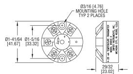
The SERIES 659 Push-Button Temperature Transmitters accept thermocouple (J, K, T), RTD (Pt100Ω) or thermistor input and provide a linearized 4 to 20 mA output. The transmitter is quickly ranged and calibrated by using a single on-board switch.
