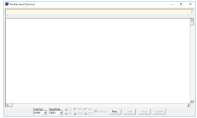
Attach your instrument & probe to your computer via the USB cable. Select the appropriate 'Com Port:'. In the below example, COM5 is being used.
