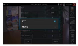
Input calling dome camera menu address code, after finishing the parameter settings, you can press the key "Enter" or click the icon call the dome camera menu.
