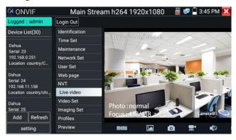
While in the "Live video" menu, click "Video Menu" at the top right of the image to access the following tools: Snapshot, Record, Photo, Playback, Lens simulation, PTZ and Settings.
