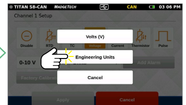
Select Engineering Units
