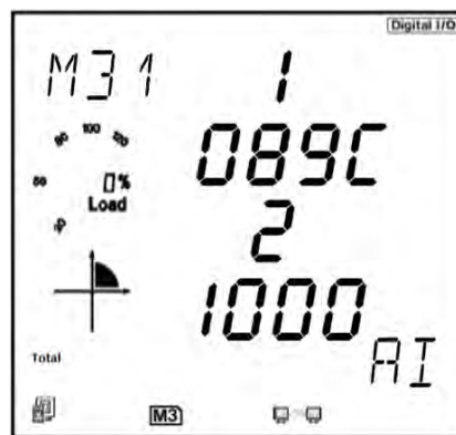
Figure 5-42 Analog Input reading from the meter display
