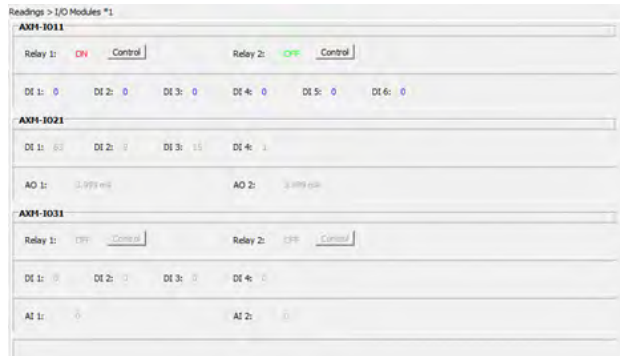
Figure 5-32 Relay Output Readings from Acuvim Software
