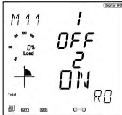
Figure 5-29 Relay Output Status Readings
