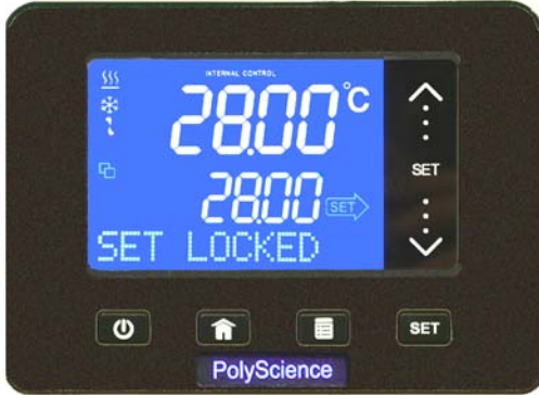
SET LOCKED – Read Commands Only Permitted
