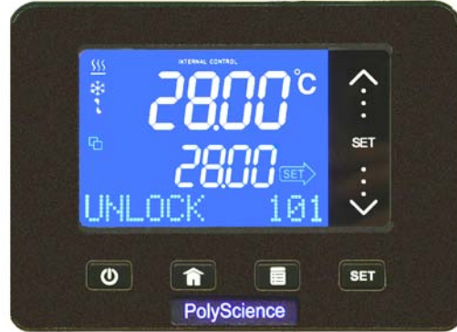
UNLOCK – Set and Read Commands Permitted
