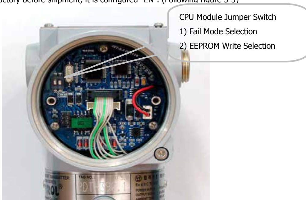
Figure 3-3. CPU Module Fail Mode, EEPROM-Write Selection Jumper Switch
