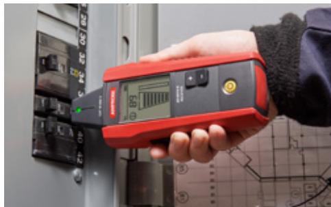
Identify the single correct breaker
