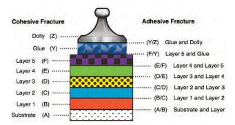
Select **Edit** to set the number of layers and cohesive/adhesive fracture details. Use the buttons to adjust.
