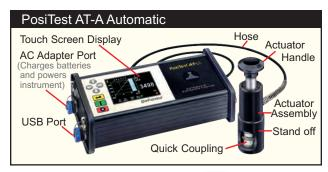
The PosiTest AT-A powers-up when the button is pressed. To preserve battery life, the instrument powers-down after 5 minutes of no activity. Alternatively, press and hold the button for 5 seconds or select Power Off from the menu.
