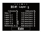
70% cohesive failure within layer 1; 30% cohesive within layer 2
