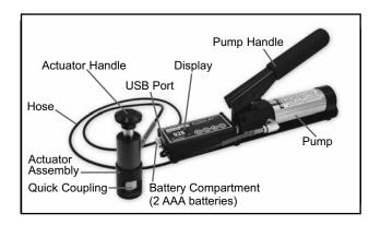
1. Ensure the pressure relief valve is completely open (turn counter clockwise)
