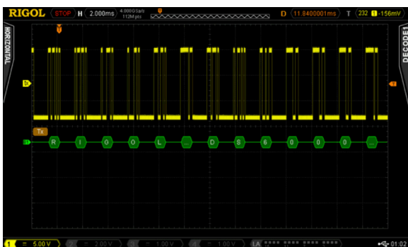
Figure 20: RS232 optimal decoded data view settings using a Rigol MSO4034Z Oscilloscope
