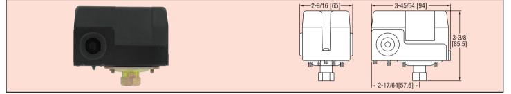
The Series CXA Water Pump Pressure Switches have been proven reliable for controlling automatic water systems. These switches are very popular for use on water pumping systems. The set point and deadband are both easily adjustable via screws inside the cover. For ease of installation, the switches come with a 1/4" female NPT process connection and can be mounted in any orientation. The series CXA's simple design makes it a great switch for an installer at any skill level.
