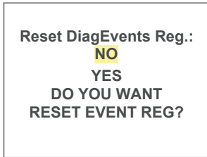
Figure 51: Resetting Diagnostic Events Register
