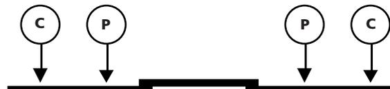
If using Duplex Handspikes ensure that the probe marked P is inside the C probes.
