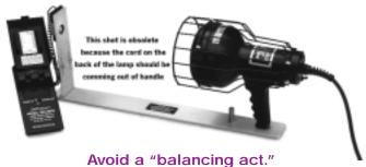
Use the Spectroline Model VF-100 Spec-Stik<sup>™</sup> MIL-STD verification fixture to calibrate your lamps at *exactly* 15 inches (38.1cm)!
