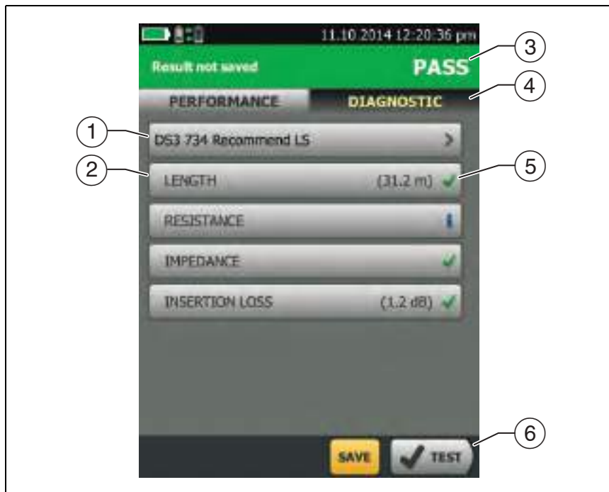
Figure 31. Autotest Results for Coaxial Cabling
