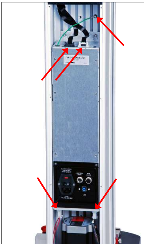
Locations of connectors and ground wire
