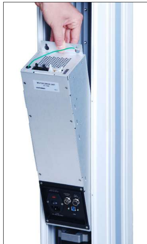
Removing the MDU
