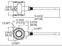
Series HHT Hazardous Area Humidity/Temperature Transmitter takes accurate measurements in the harshest of environments. The explosion-proof model fered with 4-20 mA output for humidity only. The intrinsically safe version is offered with 4-20 mA output for humidity and temperature, and do require an intrinsically safe barrier to meet hazardous area approvals.
