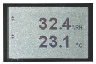
The LC display of the HP21 has a backlight which can be set to be on all the time or whenever a key is pressed. The backlight can also be disabled.
