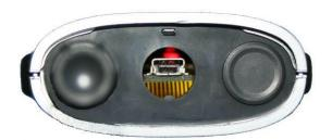
**WARNING**: the service connector is a UART interface with a mini-USB connector type. Do not connect the service connector directly to the USB port of a PC or hub.
