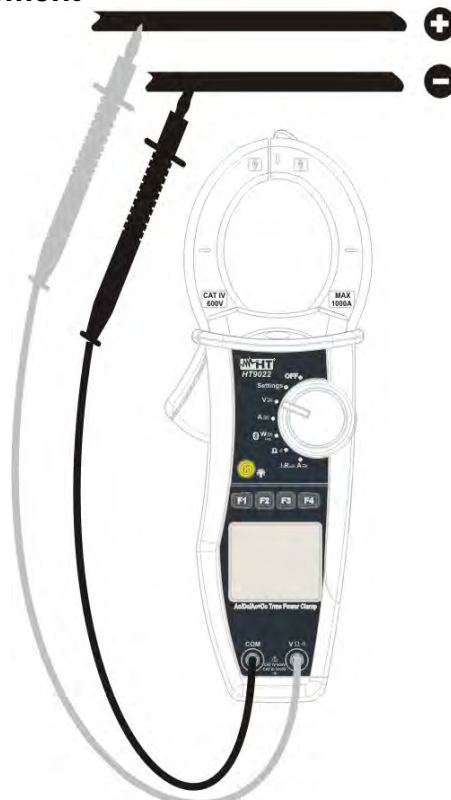
Fig. 5: DC voltage measurement
