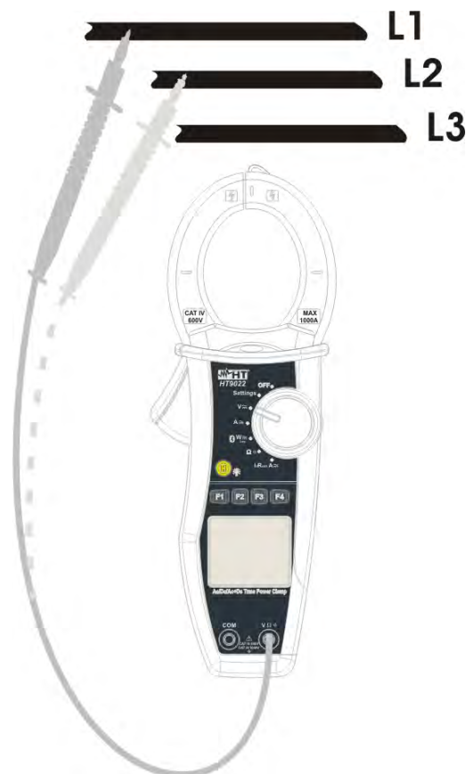
Fig. 7: verification of phase sequence
