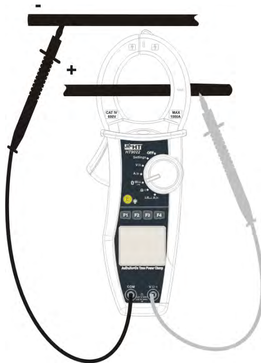
Fig. 11: DC power measurement
