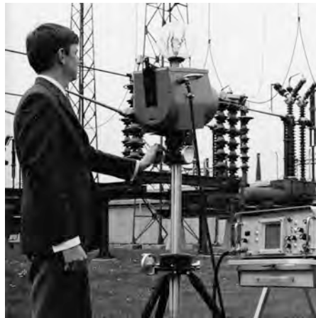
Figure 15.2 1969: Thermovision Model 661. The camera weighed approximately 25 kg (55 lb.), the oscilloscope 20 kg (44 lb.), and the tripod 15 kg (33 lb.). The operator also needed a 220 VAC generator set, and a 10 L (2.6 US gallon) jar with liquid nitrogen. To the left of the oscilloscope the Polaroid attachment (6 kg/13 lb.) can be seen.
