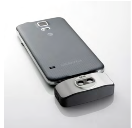
Figure 15.3 2015: FLIR One, an accessory to iPhone and Android mobile phones. Weight: 90 g (3.2 oz.).
