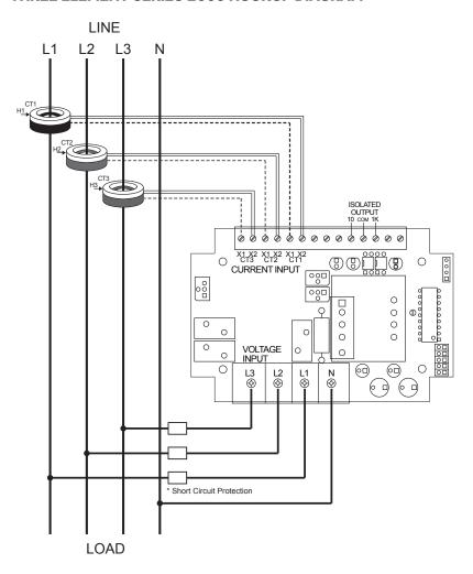
Leviton recommends solid core transformers (CTs) for revenue-grade accuracy. Our 100A and 200A color coded CTs assist with correct installation by indicating phase monitored. Split core CTs are also available upon request for applications where power cannot be interrupted during installation. Our 100-1, 200 Amp Split Core CTs offer  $\pm$ 1.0% accuracy.
